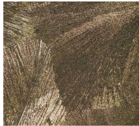
Figure 8: The coating morphology with Zn-Ni-Sn -Pb, x50
