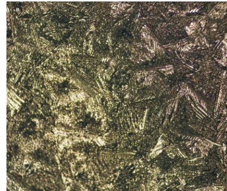
Figure 9: The coating morphology with Zn-Ni-Sn -Pb-Bi, x50
