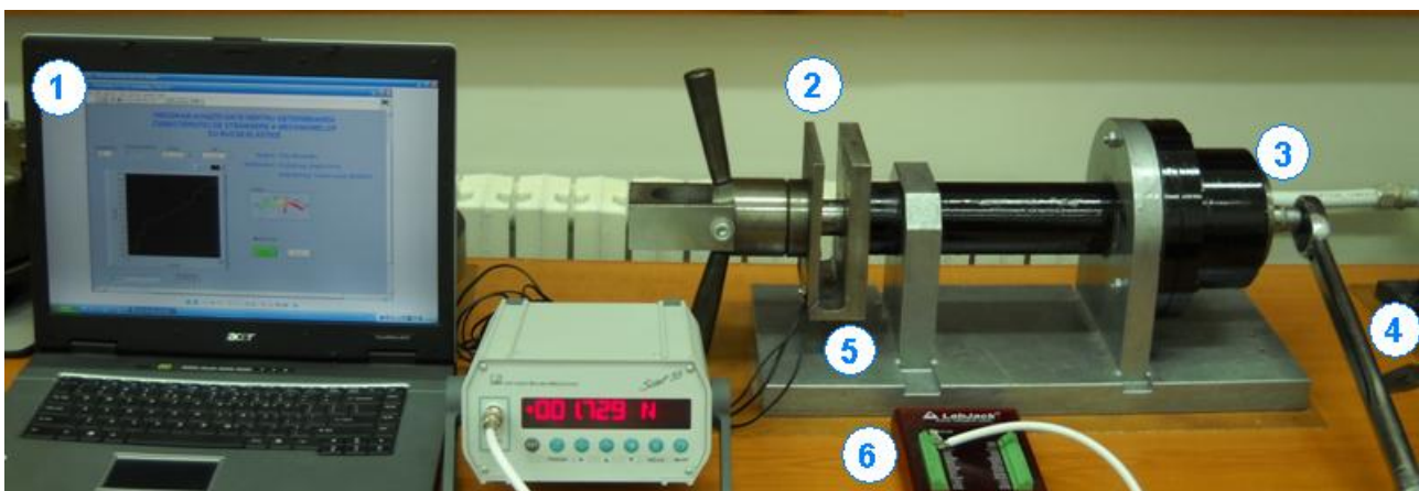
Figure 2. Structure of experiment stand, 1-computer – labview soft, 2-dynamometer, 3-chuck collet, 4-dynamometer key, 5- tensiometer bridge, 6-Labjack acquisition board
