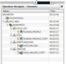
Figure 10. processing times obtained during classic simulation with NX software.
