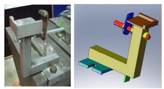
**Figure 4** – Securing device of the semi-finished attachable to the already existing stand from the robotics lab. a) real b) virtually designed in NX
