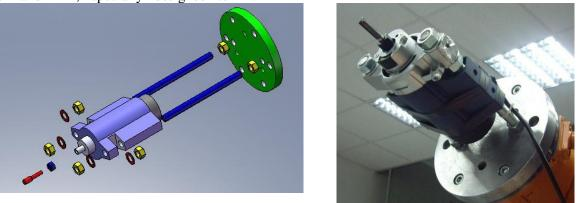
Figure 6 – Milling device attachable to the robot Kuka KR125
