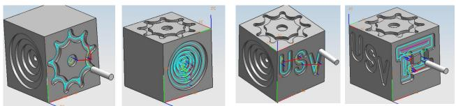
Figure 9 Simulation of classic processing on a CNC machine with the help of NX software.
