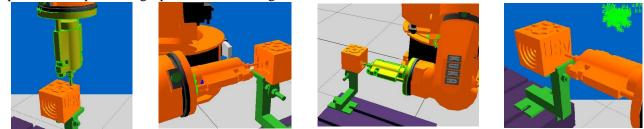
Figure 8. Simulation of form milling on cube's sides
