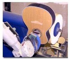
Figure 1. Details of robotics guitar buffing [11].
