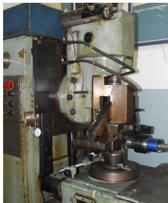
Fig. 1.4. Gear cutting machine-tool model 53A30P with the grinding device with tool disc shaped profile
