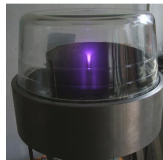
Figure 3. Installation working place during plasma discharge
