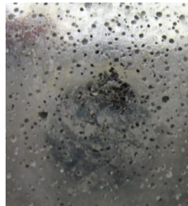
Figure 2: Macroscopic image of AlMg15 metal foam
