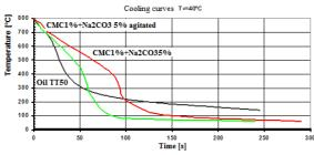
Figure 3 Cooling curves of temperature-time for different cooling environments
