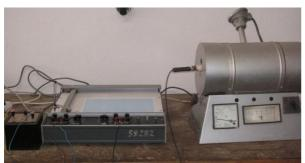
Figure 1. Image of the equipment for determination of the characteristics of cooling stage
