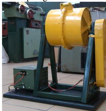
Figure 1 - Equipment for grinding metal waste (Ball mill)
