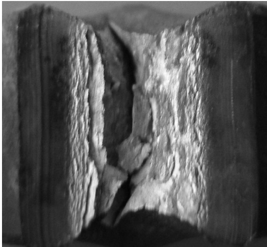
Figure 7: The heat treated stainless steel macrostructure – solution treatment 600°C aging subjected to resilience test.
