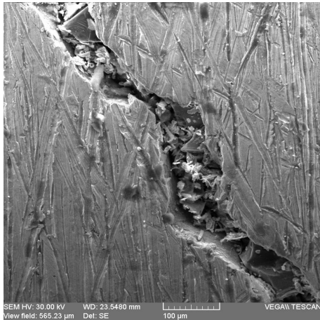
Figure 9. Microcracks on surface sample from Cu_{75.4}Zn_{18.6}Al_{5.85} alloy, magnification 500 X.
