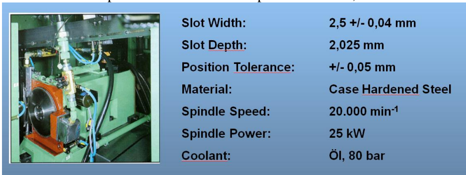
Picture 14: Grinding Data for High Speed Grinding of Pinion Grooves
