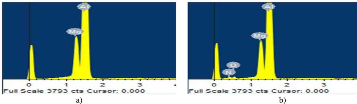
**Figure 9:** EDS analyses of the composite AlMg15/AlN (microstructures made at laboratories of Politecnico di Torino, Department of Applied Science and Technology)
