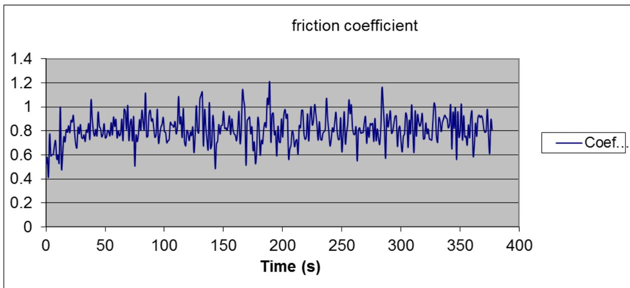
**Figure 6:** Friction wear coefficient of the AlMg10/AlN composite, value equal with 0,81428
