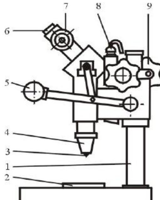
Figure 3: Microhardness machine used to determine the Vickers microhardness for AlMg/AlN composite
