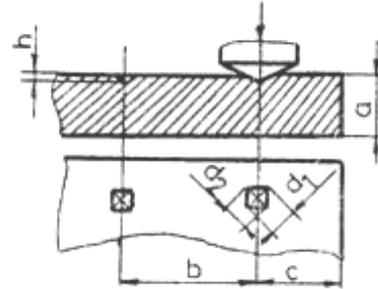
Figure 2: Scheme of microhardness test after Vickers method.
