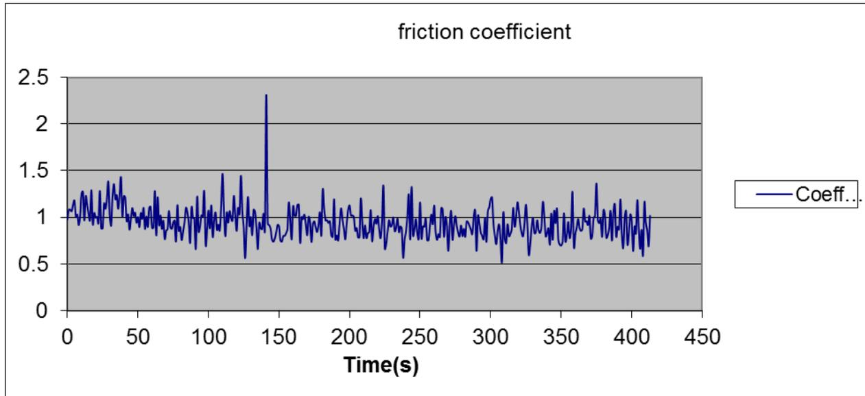
**Figure 5:** Friction wear coefficient of the AlMg5/AlN composite, value equal with 0,94622
