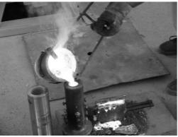
Figure 17: Casting the alloy.
