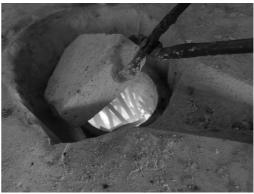
Figure 13: Melting of alloying elements.
