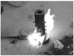
Figure 16: Shell preheating before casting alloy.
