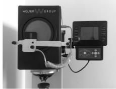
Figure 19: Wilson Wolpert universal hardness tester model 751N.
