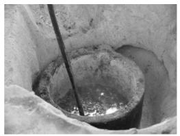
Figure 14: Homogenization of alloy.
