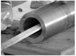
Figure 15: Metallic shell for casting alloy.
