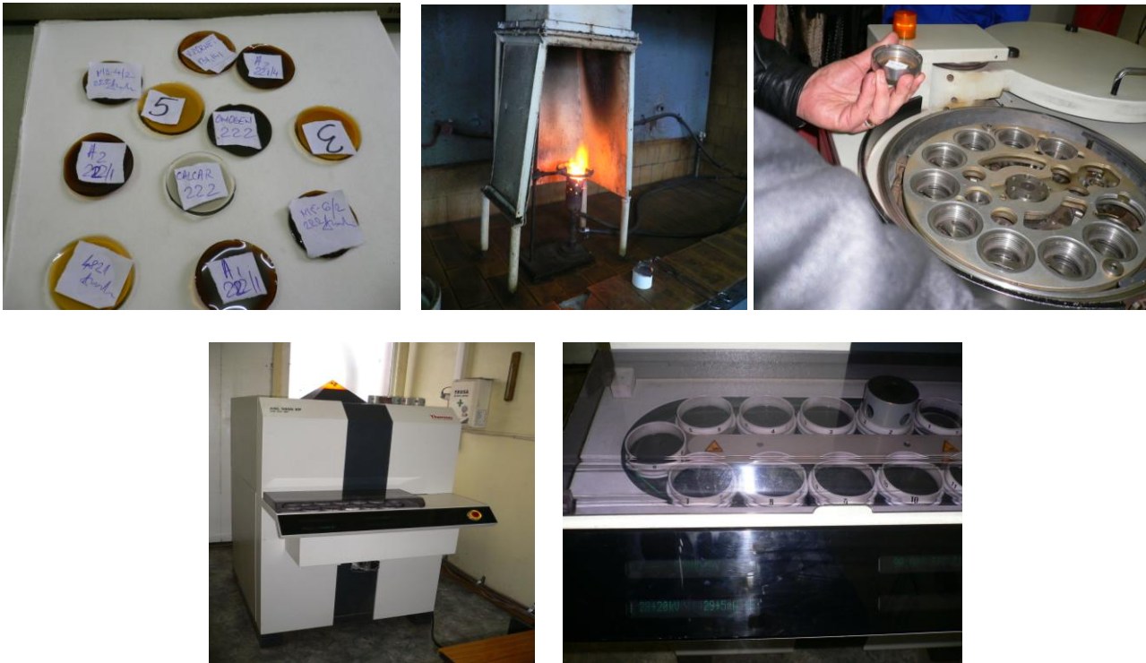
Figure 1: Preparation of homogenized samples and WD-XRF automatic analyzers used in iron and steel industry laboratories
