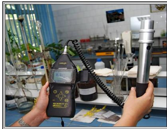
Figure7. Analyzer portable type Casella-PM10 used to capture, analysing and concentration of particulate matter.
