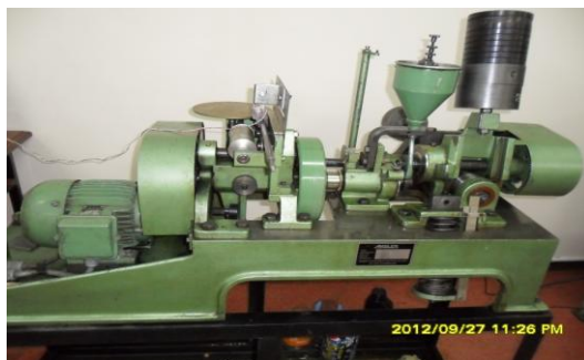
Figure 2: The AMSLER contact fatigue installation
