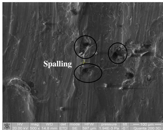
Figure 4: Multiple spalling caused by the shear stress
