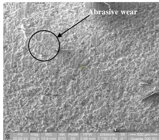
Figure 15: SEM image of the rolling surface of the deposited coating
