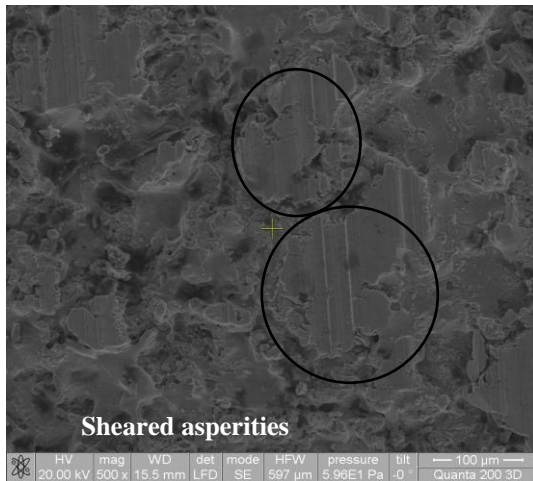
Figure 8: SEM image of the sheared asperities
