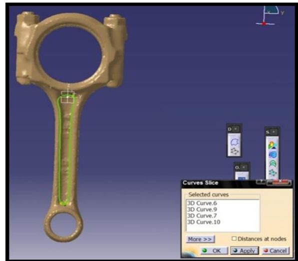
Figure 17: 3D curves merged into closed profiles.
