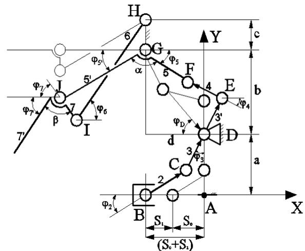
Figure 3: The mechanism of a finger.
