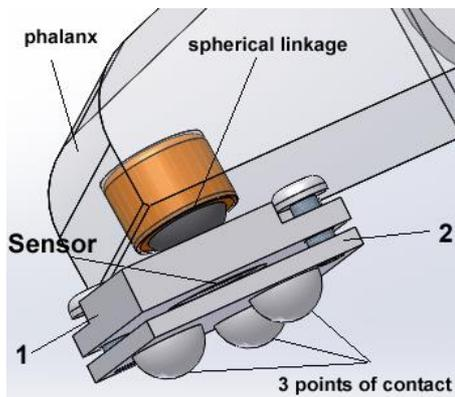
Figure 7: The jaws system, attached to the phalanxes.
