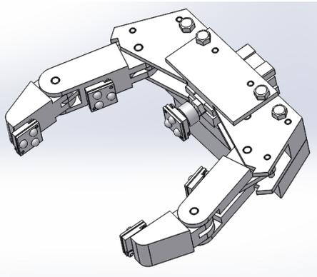
Figure 6: The two fingered anthropomorphic gripper [8].
