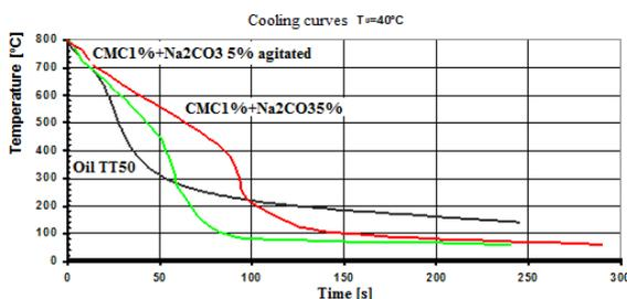
Figure 3 Cooling curves of temperature-time for different cooling environments
