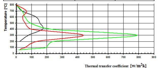
Figure 5 Coefficient of heat transfer variation depending on the temperature
