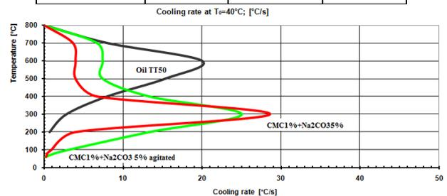
Figure 4 Chart for cooling speed variation depending on the temperature
