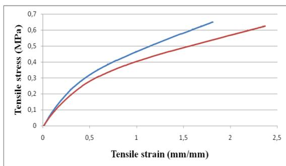
**Figure 5:** Stress-strain measurements at a strain rate of 50 mm/min (red) and 20 mm/min (blue)
