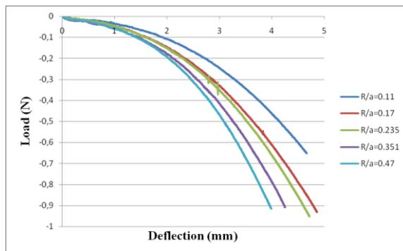
**Figure 8:** The effect of indenter size on a PDMS specimen
