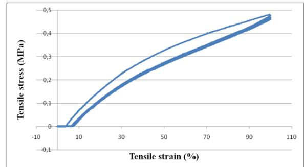
**Figure 6:** Stress relaxation data for 5 cycles at a maximum strain of 100%
