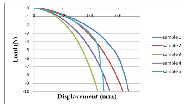
**Figure 9:** Load-displacement curves of PDMS specimens under indentation with a 8 mm spherical indenter
