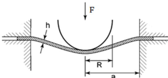
**Figure 2:** Schematic diagram of the indentation test for freestanding films [28]
