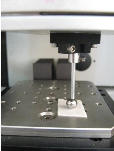
**Figure 4:** Experimental setup for indentation of flat films
