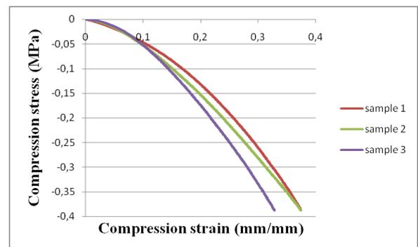
**Figure 7:** Uniaxial compressive stress-strain curves
