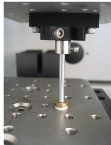
**Figure 1:** *Uniaxial compression of small PDMS circular specimens*
