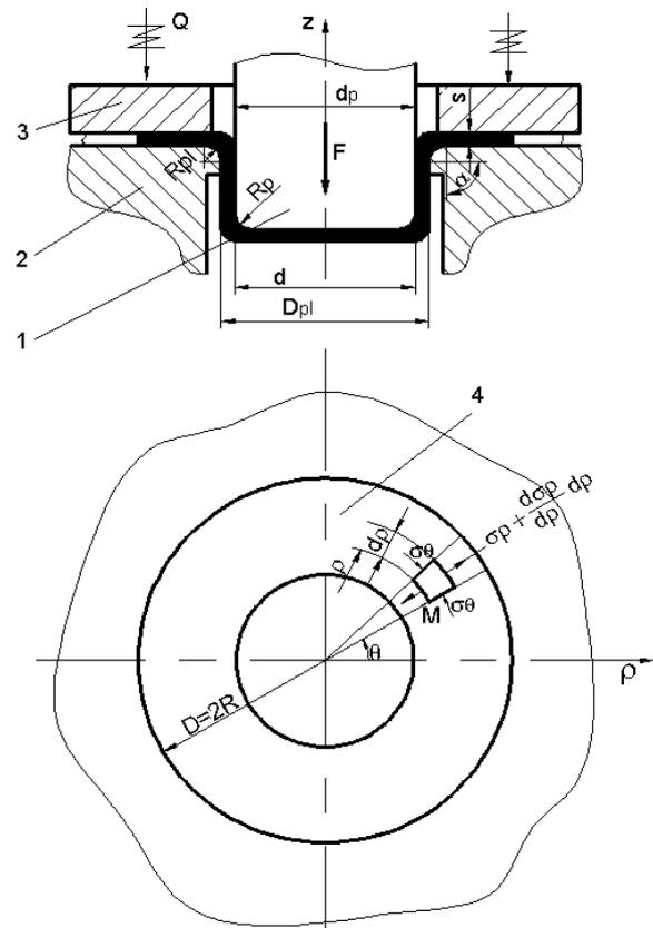
**Figure 1.** Cylindrical drawing scheme
