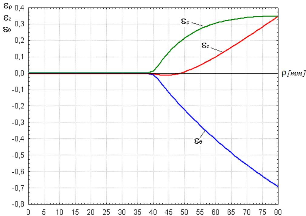
Figure 3. Graphical presentation of the real main strains along radius  $\rho$  of point  $M$  position
