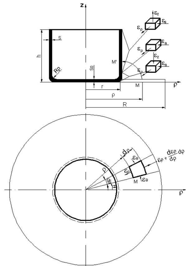
**Figure 2.** Deformation state at cylindrical drawing
