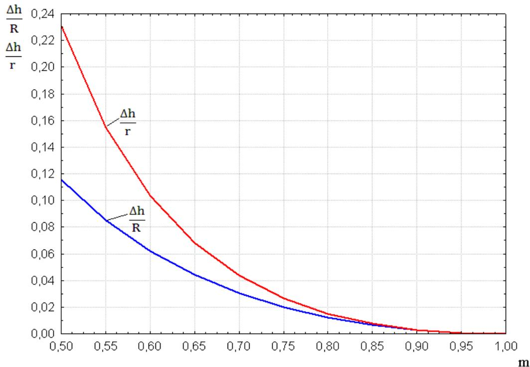
Figure 4. Graph of relative height growth of piece along drawing coefficient.
