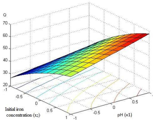
**Figure 4.** Response surface plot and contour plots for the effect of solution pH ( $x_1$ ) and Initial iron concentration ( $x_2$ ).
