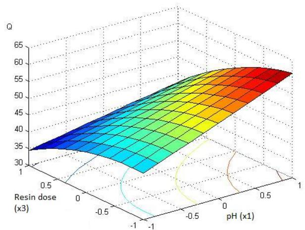
**Figure 3** Response surface plot and contour plots for the effect of solution pH ( $x_1$ ) and resin dose ( $x_3$ )
