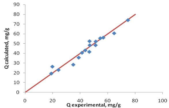
**Figure 2** Sorption capacity; experimental data versus predicted data given by regression model
