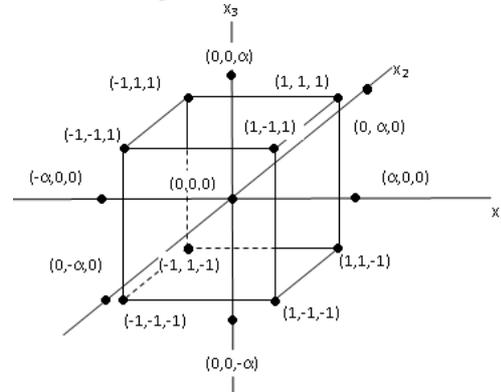
**Figure 1** Orthogonal central composite design for three independent variables and two levels [6]
