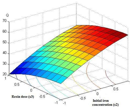
**Figure 5.** Response surface plot and contour plots for the effect of resin dose ( $x_3$ ) and initial iron concentration ( $x_2$ ).
