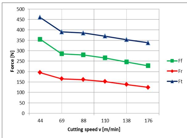
**Figure 3:** Cutting forces vs. cutting speed at  $t = 0,5$  mm and  $s = 0,2$  mm/rev
