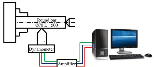
Figure 2: Set-up of the experimental study
