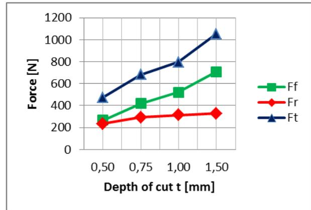
**Figure 4:** Cutting forces vs. depth of cut at  $v = 69,24$  m/ min and  $s = 0,2$  mm/rev
