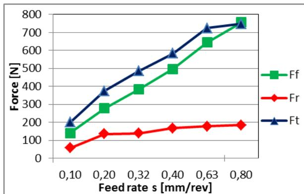
Figure 5: Cutting forces vs. feed rate at  $v = 69,24$  m/min and  $t = 1$  mm
