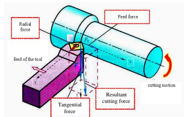
**Figure 1:** Orthogonal components of cutting force in turning [4]
