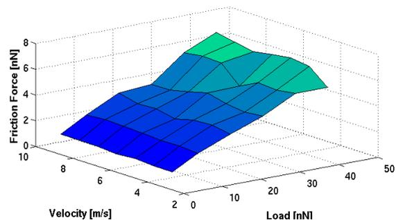
Figure 8: The friction force as a function of velocity and load
