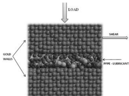
**Figure 2:** Snapshot of the simulation cell
