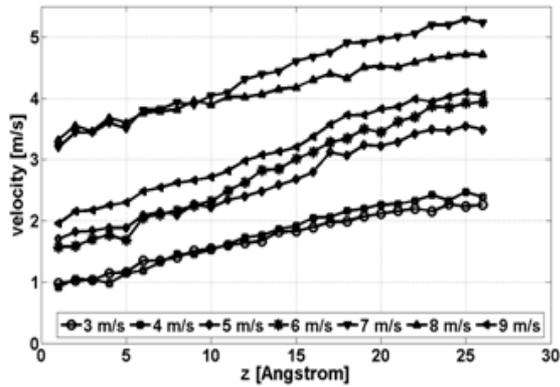
Figure 4: The velocity profile at different sliding velocities, for 1.5 GPa load
