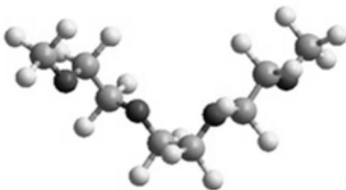
**Figure 1:** The molecular model of PFPE-Z ( $C_8F_{18}O_4$ ). Carbon atoms are gray, fluorine is white, and oxygen atoms are black.
