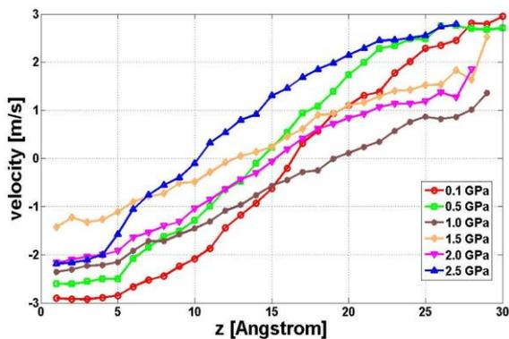
Figure 6: The velocity profile at different loads,  $v=6$  m/s
