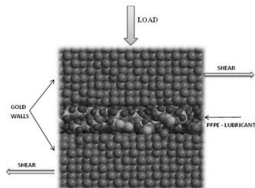
**Figure 3:** Snapshot of the simulation cell
