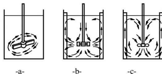
**Figure 2:** Flow pattern of mechanical rotary impellers: a) tangential; b) radial; c) axial.
