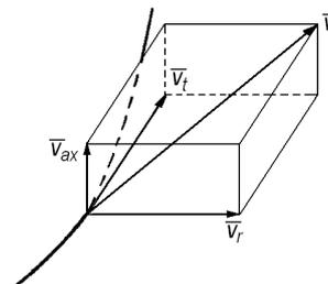
**Figure 1:** The resultant speed  $\bar{v}$  and his components:  $\bar{v}_{ax}$  - axial speed,  $\bar{v}_r$  - radial speed,  $\bar{v}_t$  - tangential speed.
