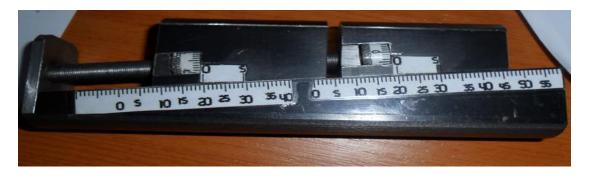
**Figure 3:** Adjustable "pass" - "do not pass" caliber with the reading system type " linear graduated scale - circular graduated vernier"
