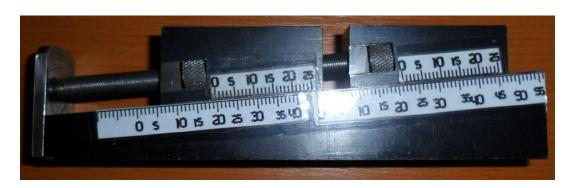
**Figure 5**: Adjustable "pass" - "do not pass" caliber with the reading system type " linear graduated scale - linear graduated vernier"
