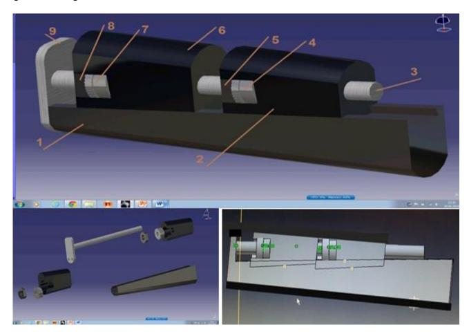
Figure 1: Adjustable limiting caliber - components
