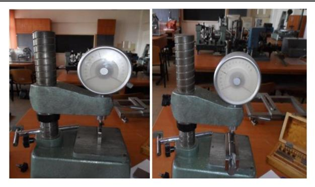
Figure 4: Adjustment to "zero" for the adjustable "pass" - "do not pass" calibers
