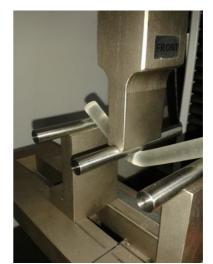
Figure 2: The bending specimen sample.
