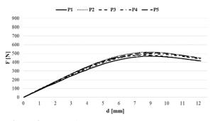
Figure 3: Force-dispacement curve for epoxy Resin.
