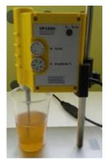
Figure 1: Ultrasonic Processor UP100H during epoxy treatment.
