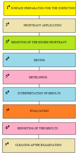
Figure 2: Steps of liquid penetrant inspection
