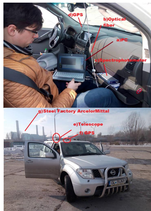
Figure 2: The UGAL mobile DOAS system
