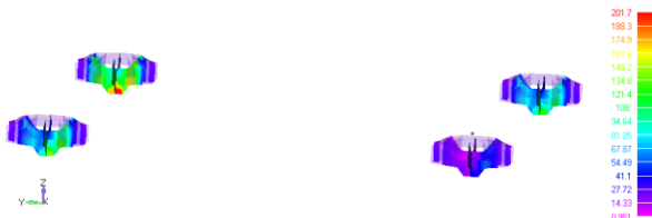
Figure 16: Von Mises stress for spudcan for LC2 (elevated condition)
