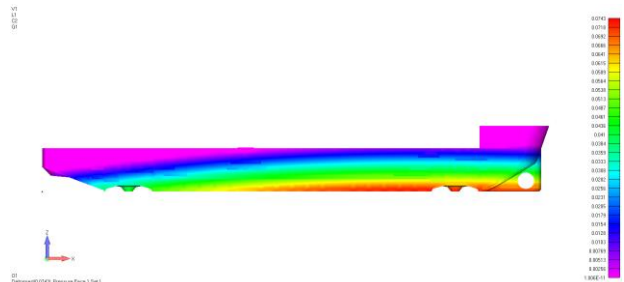
Figure 9: External hydro pressure loads – trim and wave amid ship
