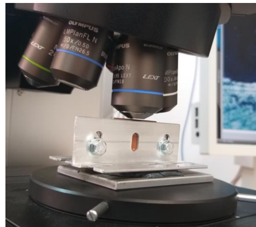
Figure 1 Positioning the sample on the table of the Olympus LEXT OLS4100 laser microscope
