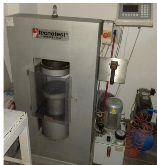
Figure 2: The concrete testing machine with KL 300/CE dual piston KL 300/CE.
