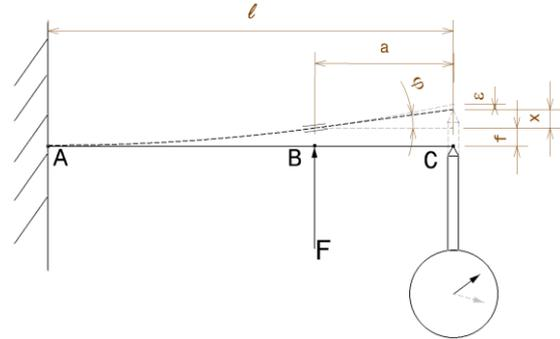
Figure 2 : Loading scheme of the elastic lamella
