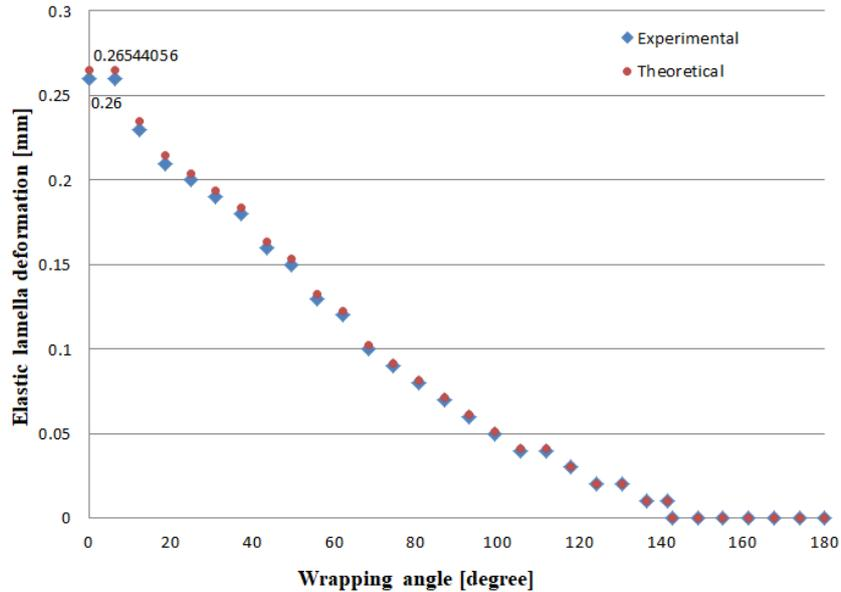
Figure 3 : Theoretical and experimental deformation values of lamella when loading with mass of 0.74 Kg
