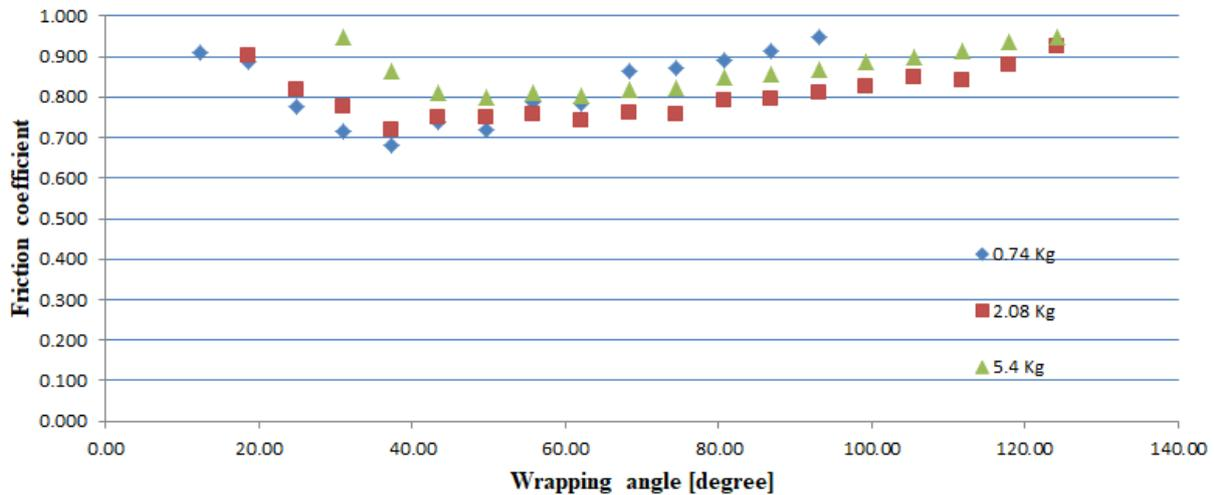
**Figure 5** : Friction coefficient dependence with wrapping angle
