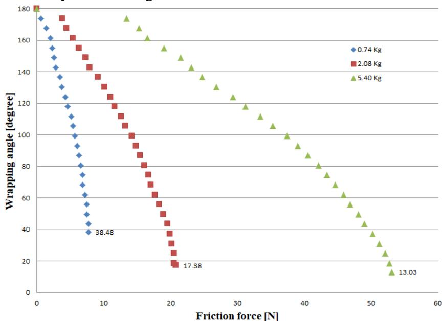
**Figure 4** : Evolution of the slipping angle with the load
