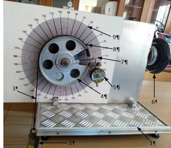
Figure 1 : Components of the experimental device
