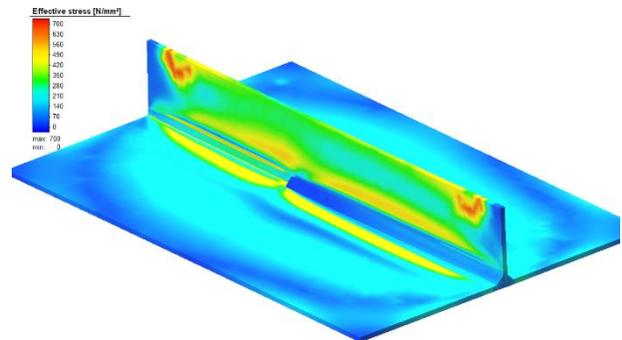
**Figure 12:** The Von Mises stresses distribution in plate at 9.5s
