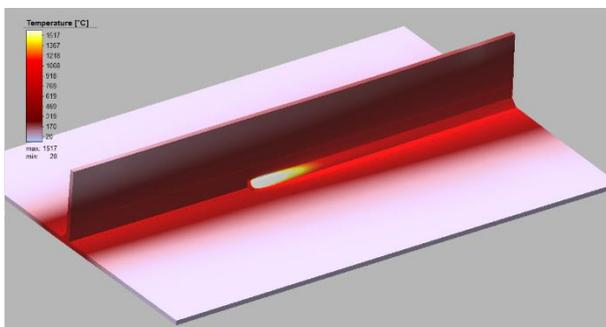
Figure 4: Thermal field at 9.5s
