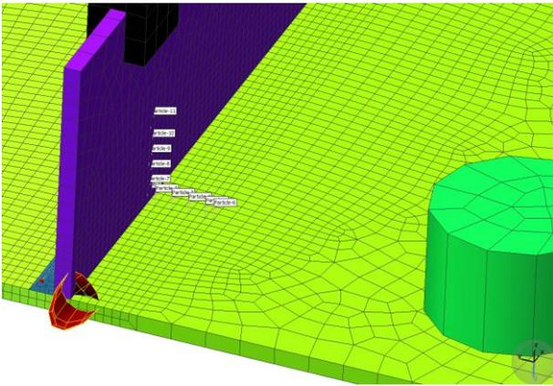
**Figure 8:** Selected nodes in deck and web plates for monitoring the temperature and stresses
