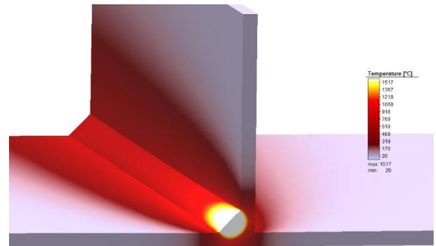
Figure 5: Cross section through the molten metal pool at 3.5s
