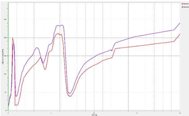
Figure 14: Effective stress in nodes of the web plate
