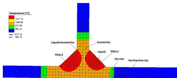
Figure 7: Phase fractions in two moments during welding
