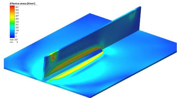
**Figure 11:** The Von Mises stresses distribution in plate at 3.5s
