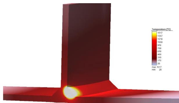
Figure 6: Cross section through the molten metal pool at 9.5s
