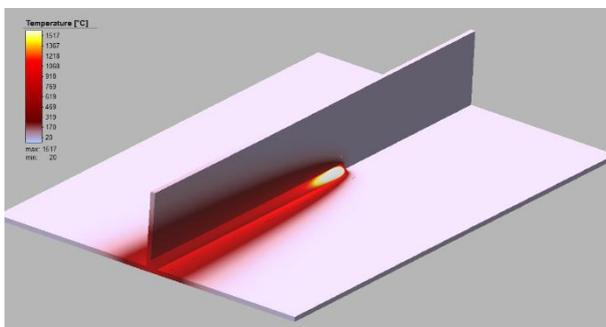
Figure 3: Thermal field at 3.5s
