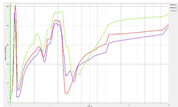
**Figure 13:** Effective stress in nodes of the deck plate
