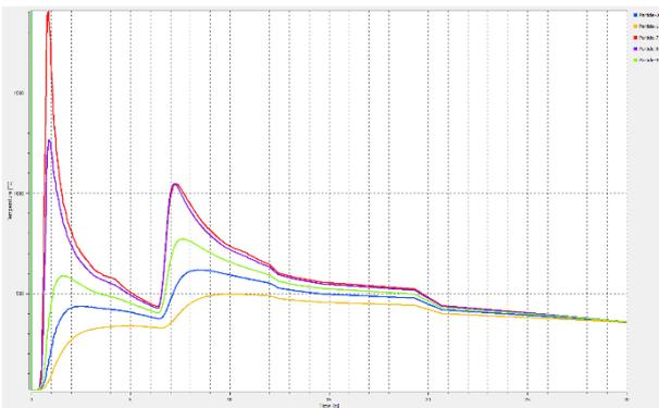
**Figure 10:** Thermal cycle in nodes of the web plate
