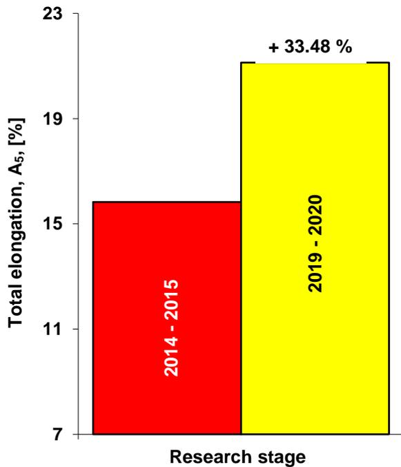
**Figure 5:** The total elongation ( $A_5$ ) of dual-phase steel depending on the research stage.
