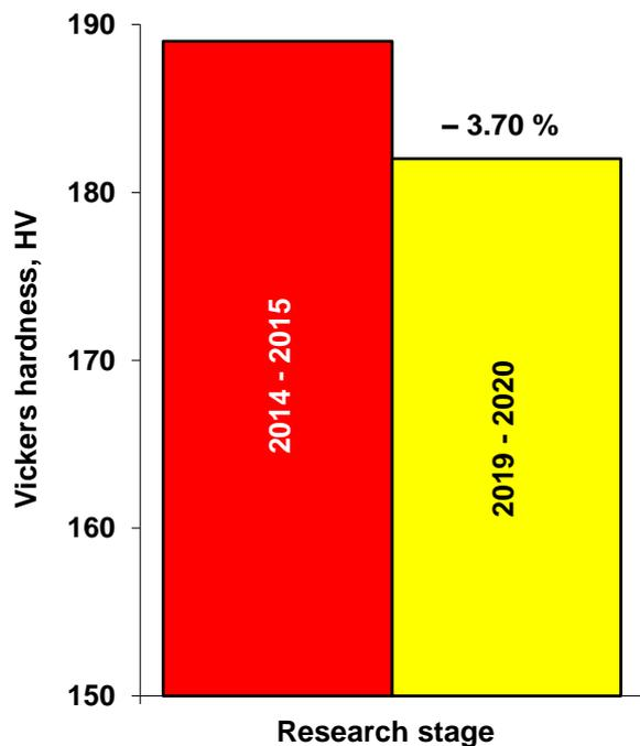
**Figure 6:** Vickers hardness (HV) of dual-phase steel according to the research stage.
