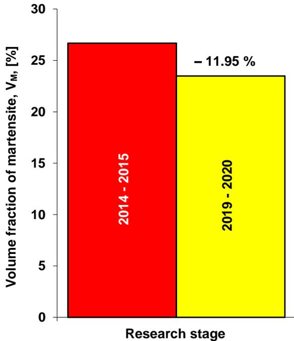
**Figure 3:** The volume fraction of martensite ( $V_M$ ) in the structure of dual-phase steel according to the research stage.
