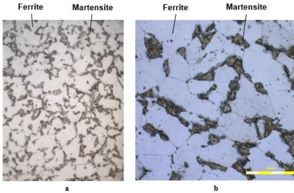
**Figure 2:** Ferrite-martensite structures
