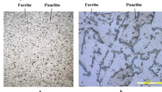
**Figure 1:** Ferrite-pearlite structures
