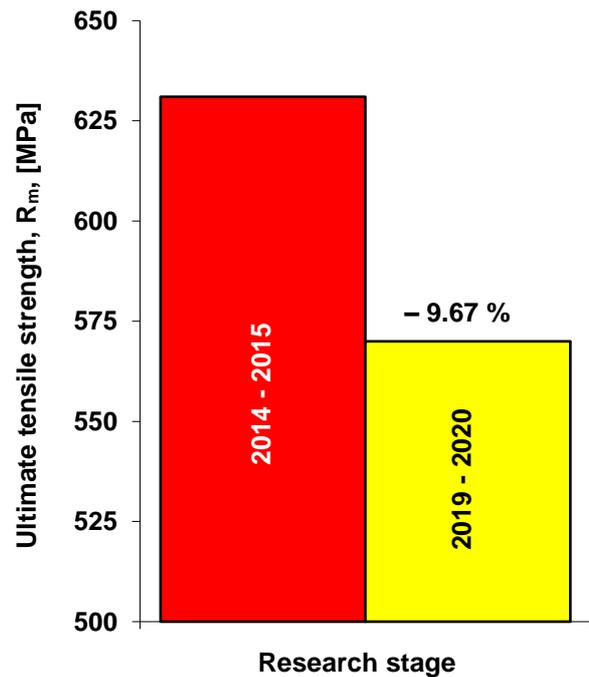
**Figure 4:** The ultimate tensile strength ( $R_m$ ) of dual-phase steel depending on the research stage.
