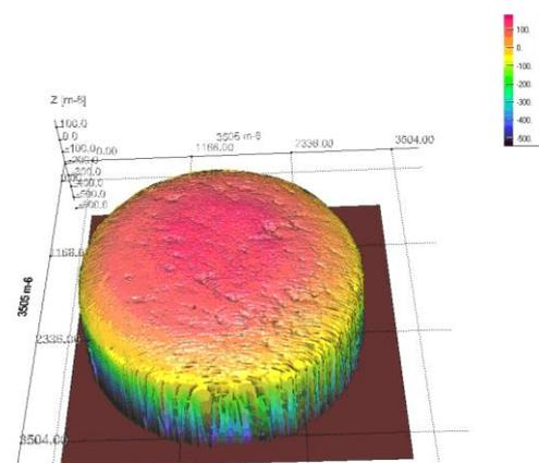
**Figure 5:** 3D surface representation for a new spark plug with dual lateral electrode configuration
