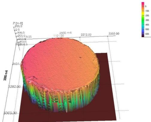
**Figure 2:** 3D surface representation for a new spark plug with single lateral electrode configuration
