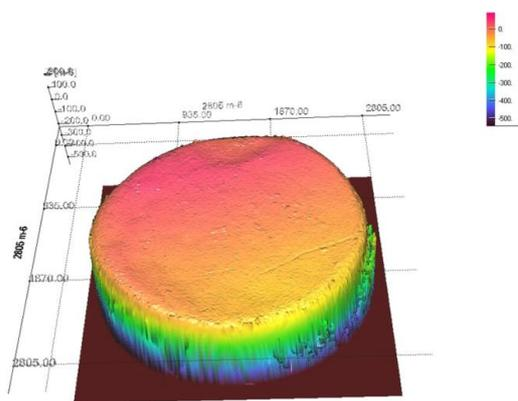
**Figure 3:** 3D surface representation for a worn out spark plug with single lateral electrode configuration
