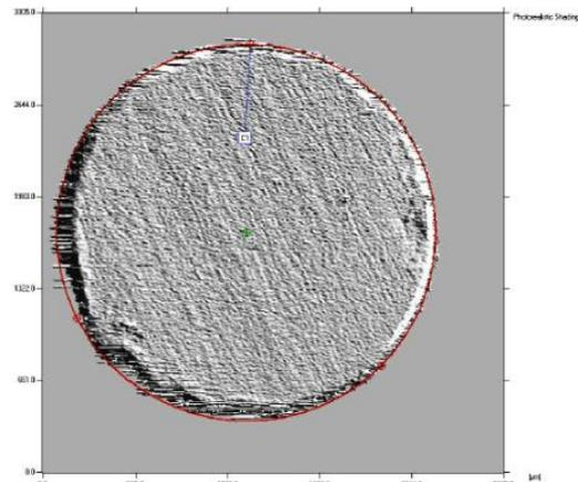
**Figure 13:** Sample plane representation and circumference measurement of the central electrode for a single electrode spark plug configuration
