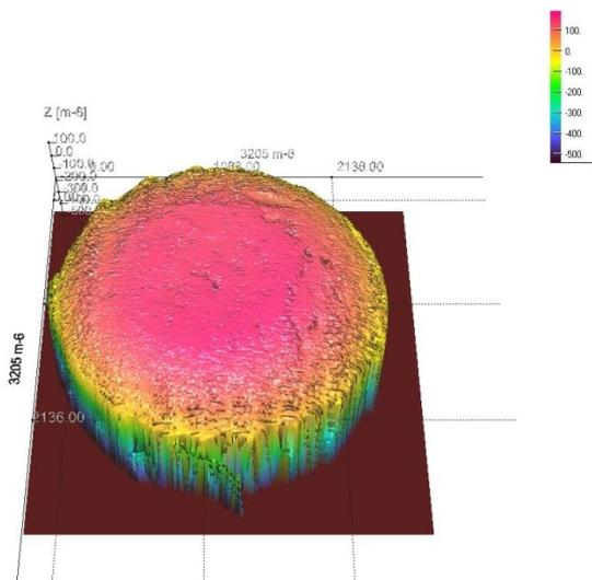
**Figure 11:** 3D surface representation for a new spark plug with four lateral electrodes configuration
