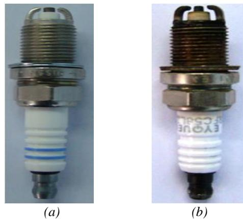
**Figure 4:** New (a) and worn (b) spark plug with dual lateral electrode
