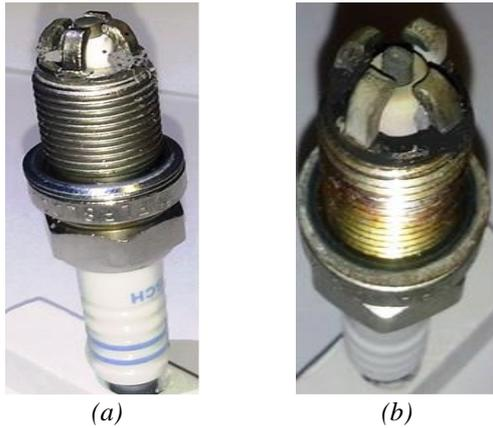
**Figure 10:** New (a) and worn (b) spark plug with quadruple lateral electrode
