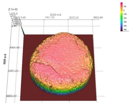
**Figure 9:** 3D surface representation for a worn out spark plug with triple lateral electrode configuration
