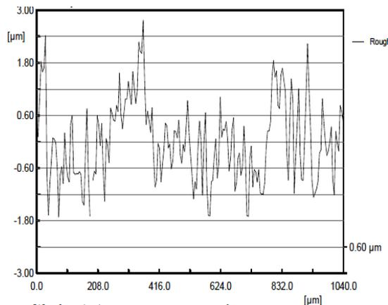
**Figure 14:** Sample roughness profile representation for a single electrode spark plug configuration
