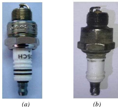
**Figure 1:** New (a) and worn (b) spark plug with single lateral electrode
