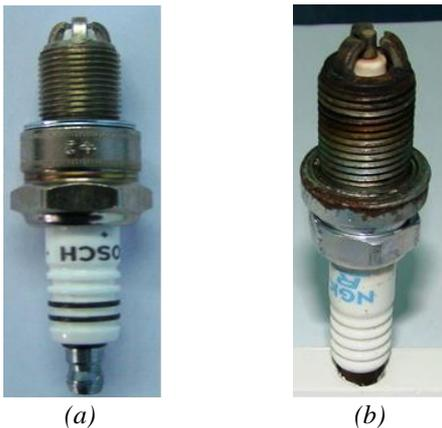
**Figure 7:** New (a) and worn (b) spark plug with triple lateral electrode
