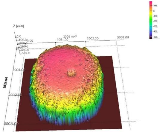
**Figure 6:** 3D surface representation for a worn out spark plug with dual lateral electrode configuration
