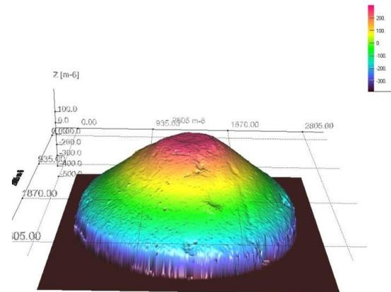
**Figure 12:** 3D surface representation for a worn spark plug with four lateral electrodes configuration
