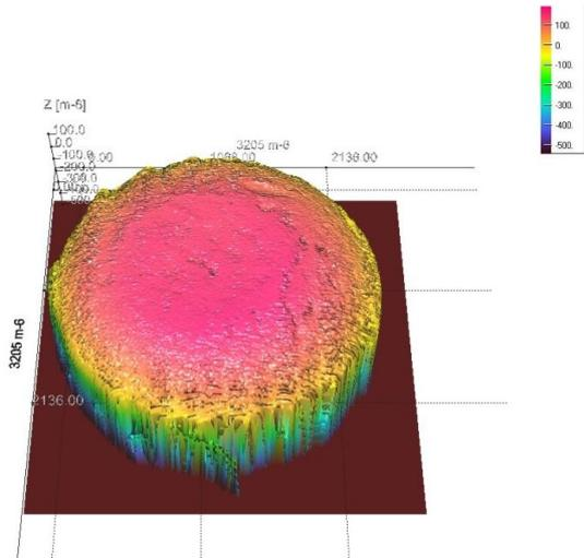
**Figure 8:** 3D surface representation for a new spark plug with triple lateral electrode configuration
