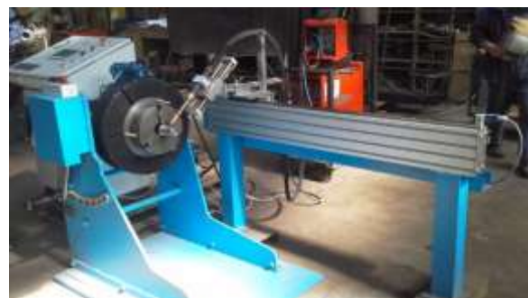
Figure 2: Appearance of the CNC system with rotary and linear modules and control panel visible on the left.
