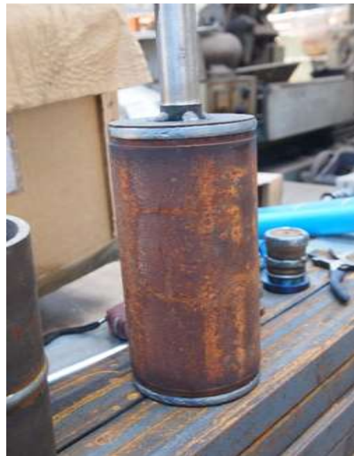
Figure 11 (a), (b): Welding plugs to a cylinder
