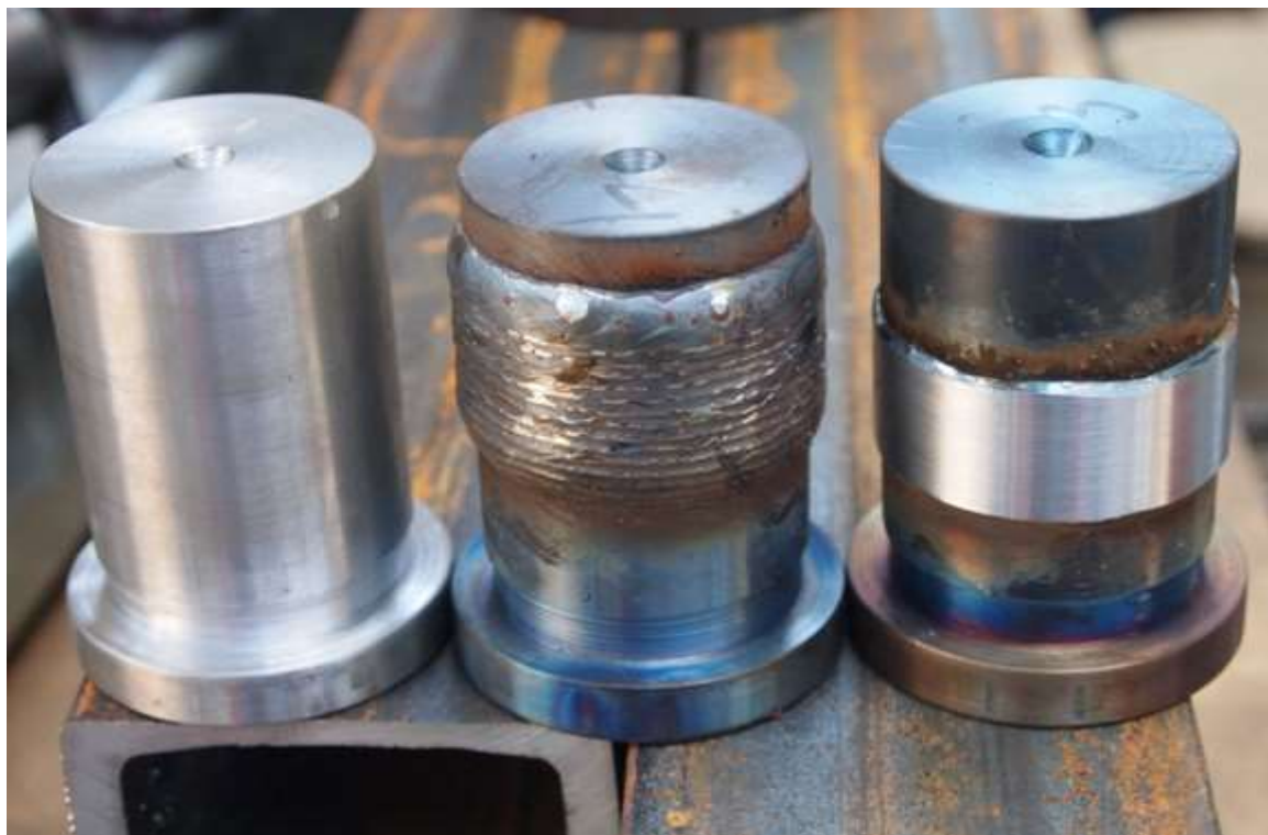
Figure 12: Workpieces subjected to overlay welding using the modular complex: a – the piece is subjected to mechanical processing before overlay welding; b – the piece is overlay welded using the modular complex; c – the piece after finishing mechanical processing.
