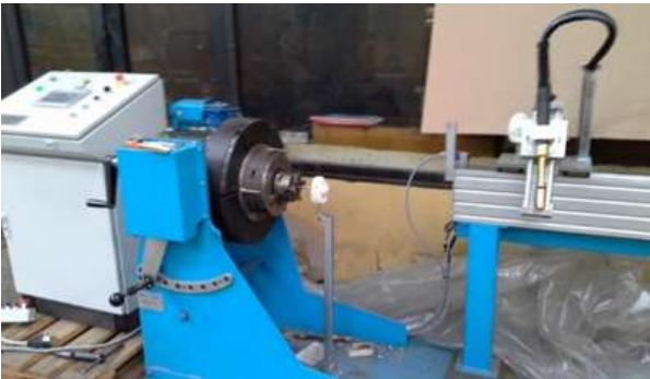
Figure 3: Optical coding device connected with the main axis of the sensor
