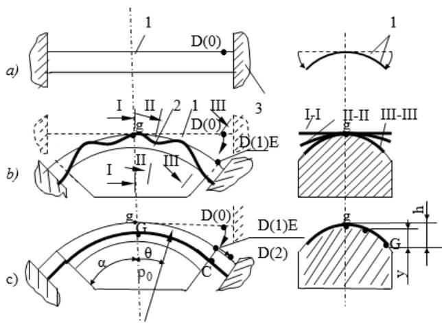
**Figure 4.** Succession of bending with tension on biconvex surfaces
