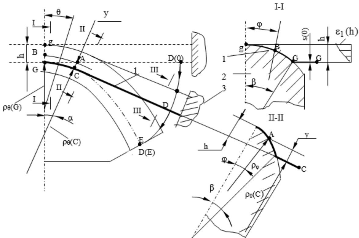
**Figure 2.** Diagram of the extension of the wide strips on the punch with biconvex surface 1-semi-finished; 2-punch; 3-clamping device
