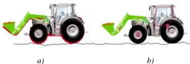
Figure 6. Implementation of Boom Suspension system for reducing the balance of the loaded bucket [Fendt]: a) without system; b) with system.
