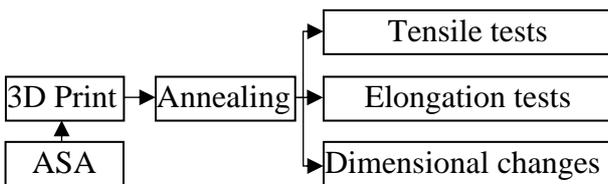
Figure 1: Experimental plan
