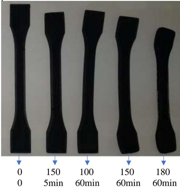
**Figure 7:** Dimensional variation of annealed ABS test specimens
