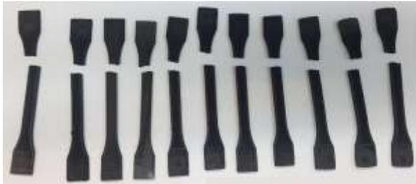
a. Fracture location for all test specimens
