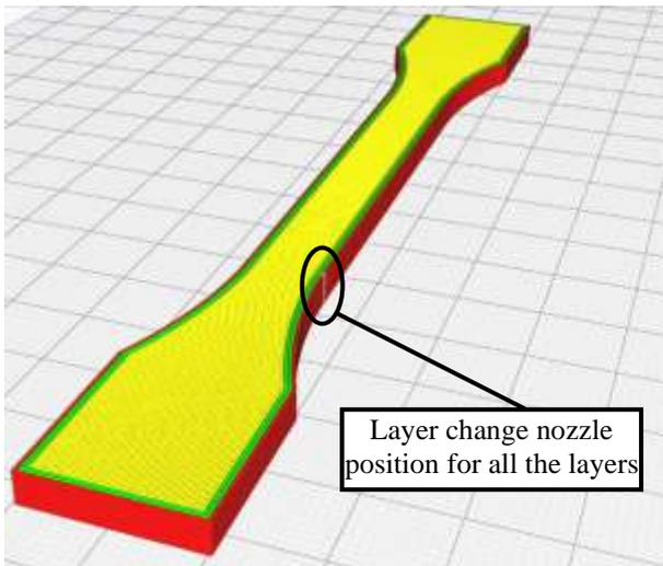
**Figure 4:** Layer change positioning
